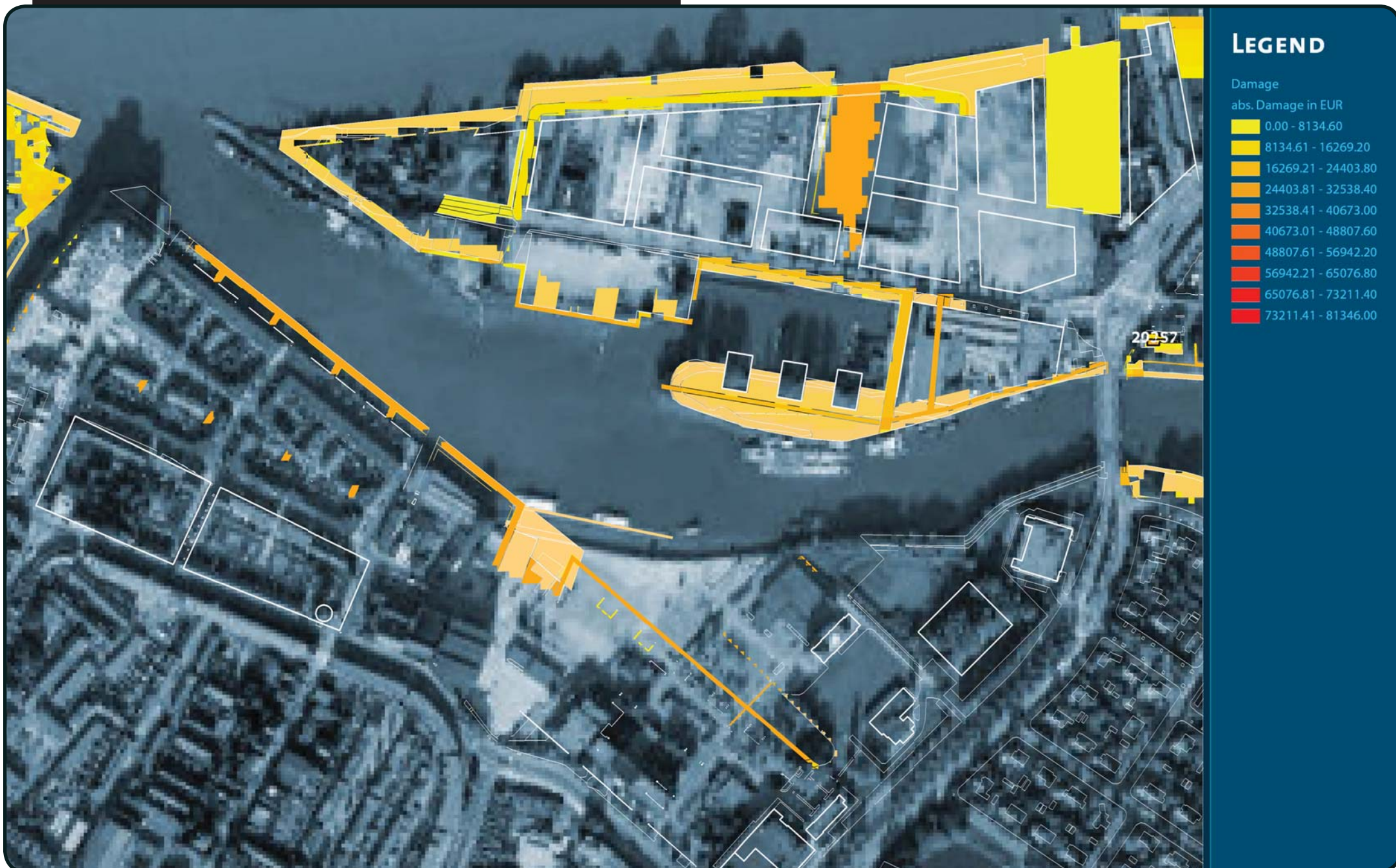
Fig 2: Expected damages for a 2000 year flood on the Waterstairs design
